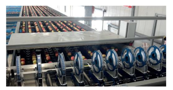
System for bulk labeling, designed to be used for sizer and roller bench labeling, particularly flexible and adaptable to other components and existing devices. The system functions thanks to an interface connection in the case of the sizer, or with a fruit presence photocell in the case of the roller bench.
